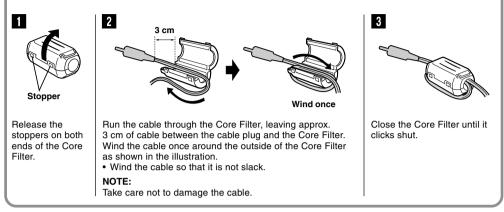
• When connecting cables, attach the end with the Core Filter to the camcorder.
